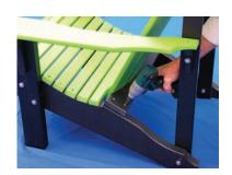
**Step 6** - Fasten bottom of back to seat assembly with two 2" screws in each side.
