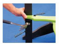
Step 3 - Fasten back legs to armrests with a 2½" bolt, two washers, and a nut.
