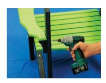
**Step 4** - Fasten back legs to armrests with a 2" screw in each leg.
