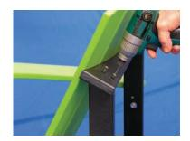
**Step 7** - Fasten ledge at top of back assembly to top of back legs with two 2" screws in each leg.
