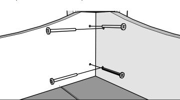
2. Assemble (B)- Legs to (A) Top as shown using 4 - 1 1/2" Screws per leg :Note: Make sure that (A) top & (B) legs are positioned as in picture below.
