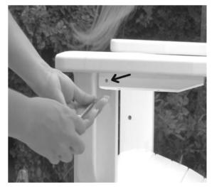
Put the head of the bolt on the inside so that the threads of the bolt are on the outter side of the leg.
