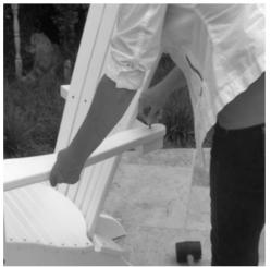
Rest the front part of the arm on the front leg while connecting the back of the arm to the back.
