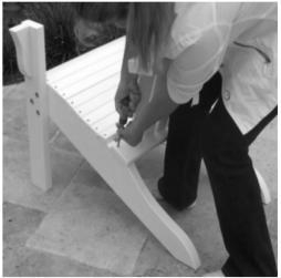
Make sure to have the bottom of the back push up against the back of the seat. Screw directly into the material on the top of the leg.
