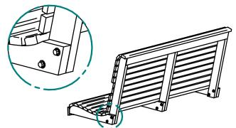
2. Attach Armrest Assemblies to each side using 3 1/2" Bolts in front hole.
