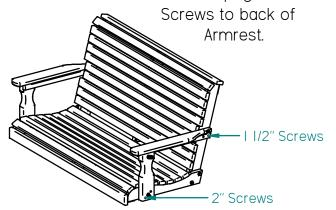
5. Attach short end of Chain to Back and other end through screw eye to bottom of
