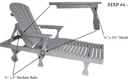
First assemble the arm assembly using 1/4" x 23/4" machine bolts and one washer. Then fasten the arm assembly to the seat support and the back using 1/4" x 3" machine bolts and washers. (See motion point diagram.)
