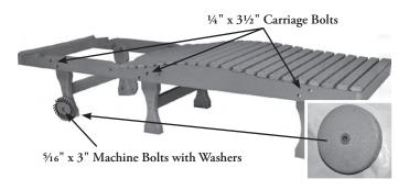
STEP #1 -Fasten the three leg assemblies to the seat using 1/4" x 31/2" carriage bolts. Then attach the wheel using 5/16" x 3" machine bolts and washers. (See motion point diagram.)
