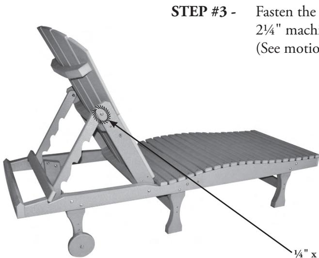
**STEP #3 -** Fasten the reclining brace using  $\frac{1}{4}$ " x  $2\frac{1}{4}$ " machine bolts with two washers. (See motion point diagram.)
