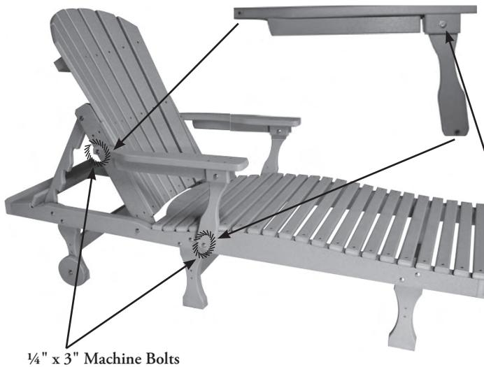
**STEP #4 -** First assemble the arm assembly using  $\frac{1}{4}$ " x  $2\frac{3}{4}$ " machine bolts and one washer. Then fasten the arm assembly to the seat support and the back using  $\frac{1}{4}$ " x 3" machine bolts and washers. (See motion point diagram.)
